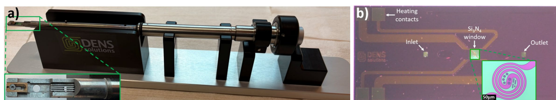
Figure 17. a) DENSsolutions single tilt heating holder. The insert shows the holder tip. b) In situ (gas, bottom) chip. Different elements of the chip are indicated. The insert shows a zoomed in image of the \text{Si}_3\text{N}_4 window.
