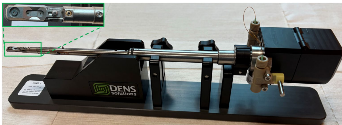
Figure 18. DENSsolutions Climate in situ (gas) holder. The insert shows the holder tip.
