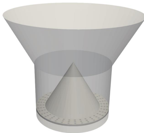
Figure 6-1 Proposed reactor geometry for follow up studies. Including a distributor plate with a central cone and a wider section right above the top of the cone.
