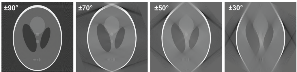
Figure 1.16: Effect of the missing wedge for the Shepp-Logan phantom. The tilt range is indicated in the figures. The final reconstruction is blurred and elongated.
