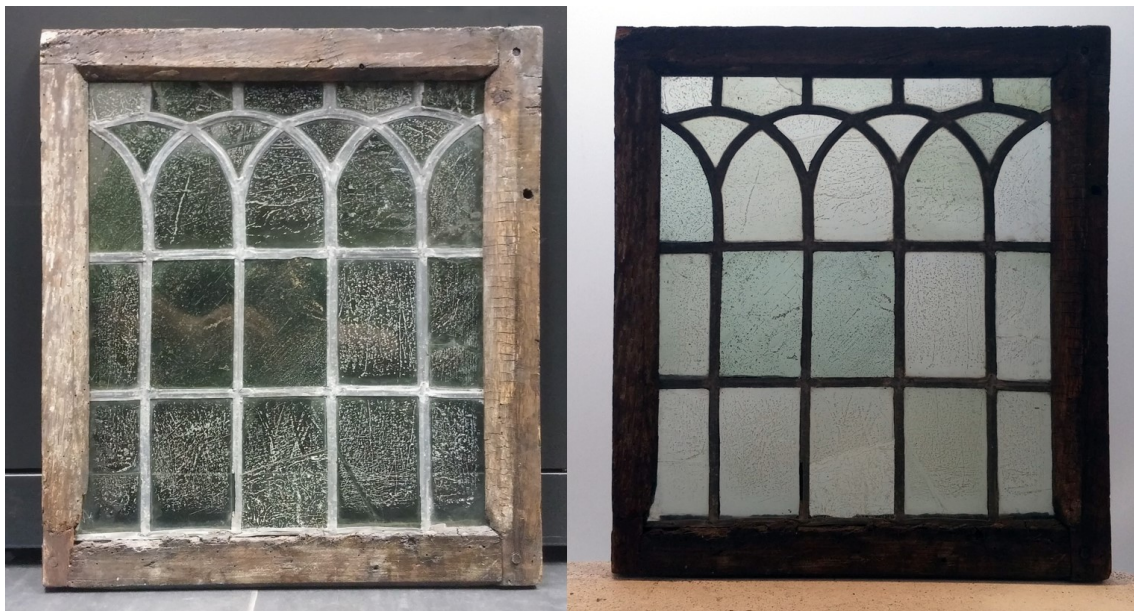
Figure 1. Visual light images of the interior side of the inspected window in reflected ( left ) and transmitted light ( right ).
