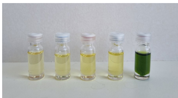
Fig. 5 From left to right: pure linseed oil, linseed oil with 5 wt.% of zinc oleate, with 5 wt.% of Pb oleate, with 5 wt.% of Ca oleate, and 5 wt.% of Cu oleate
