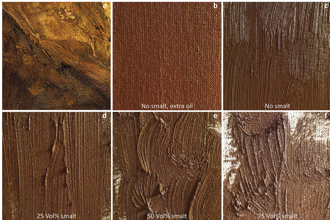
Fig. 8 Detail of brushwork in Homer's sleeve (a) and a series of paint reconstructions applied with a brush showing the effect of different volume percentages of smalt on the surface texture of the paint: mixture of red earth, yellow earth and a little bone black, diluted with oil (b), mixture of red earth, yellow earth and little bone black (c), same pigment mixture as (c) with 25 volume% smalt (d), with 50 volume% smalt (e), with 75 volume% smalt (f)
