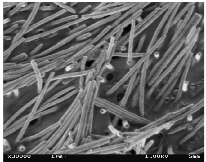
FIG. 1. Scanning electron microscopy–field emission gun micrograph of lead nanowires after dissolution of the hosting polycarbonate membrane with dichloromethane.
