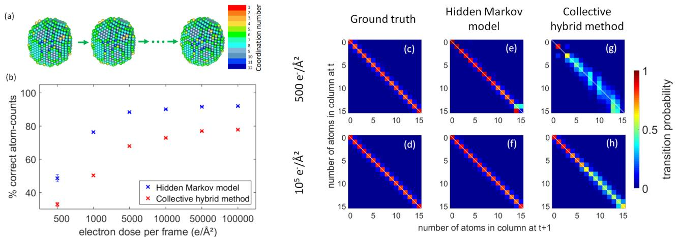
Figure 2. (a) Example of the 3D atomic structure of the changing Pt nanoparticle. (b) Percentage of correctly counted atomic columns, with a 95% confidence interval as a function of the electron dose in each individual frame. (c)-(h) Ground truth and estimated transition matrices using the hidden Markov model analysis and the collective hybrid method with electron dose  $5 \times 10^2$  and  $10^5 e^-/\text{\AA}^2$ .
