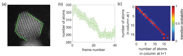
Figure 4. (a) The Pt nanoparticle shows clear facets along the beam direction. Atomic columns in  $\{111\}$  facets are indicated. (b) Number of atoms in the  $\{111\}$  facets indicated in (a). (c) Estimated transition probability matrix.
