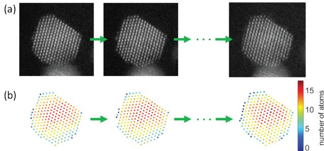
Figure 3. (a) The experimental ADF STEM time series of a Pt nanoparticle. (b) From the estimated hidden Markov model, the hidden state sequence is retrieved.
