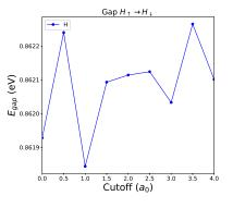
FIG. 3: The defect gap maximization for the interstitial tetrahedral hydrogen defect in diamond using the conventional DFT- $\frac{1}{2}$  method.
