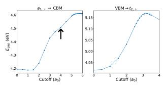
FIG. 8: The maximization of the gaps  $E_{VBM \to unocc}$ and  $E_{occ \to CBM}$  for the absorption energy of the V(-)center. An arrow was added to the  $E_{occ \to CBM}$  curve to highlight the kink in the curve.
