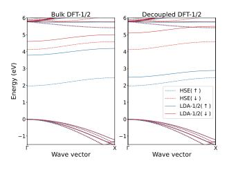
FIG. 6: The band structure of tetrahedral hydrogen for a  $2 \times 2 \times 2$  diamond conventional supercell using bulk DFT- $\frac{1}{2}$  and HSE06 (left) and bulk+decoupled, DFT- $\frac{1}{2}$ and HSE06 (right). The zero point of energy was set at the VBM for all calculations.
