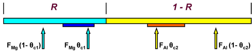
Figure 2. Schematic picture of the deposition process used in the analytical surface model. Sputtered metal fluxes arriving at the substrate are shown as blue (Mg) and yellow (Al) arrows. Note that the oxidized parts of the substrate are shown in darker blue (MgO) and orange colors ( \text{Al}_2\text{O}_3 ). R is the Mg metal ratio ( R = N_{\text{Mg}}/(N_{\text{Mg}} + N_{\text{Al}}) ).
