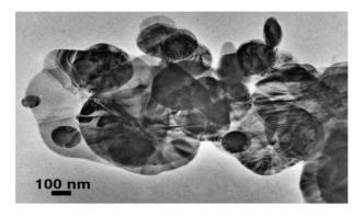
Figure 2. A TEM image of an aggregate of h-BN crystallites viewed along the [0002] zone axis.
