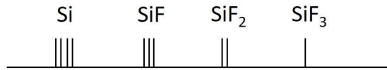
Figure 20. Schematics of the bonds between a Si substrate and (from left to right) a Si_{(s)} , SiF_{(s)} , SiF_{2(s)} and SiF_{3(s)} group. The unfluorinated Si atom is attached to the material with three strong Si-Si bonds and a weak one, making its total bond strength approximately equal to the one of the SiF group. The SiF_{2(s)} group is attached less strongly to the surface due to its lower number of bonds. The single bond of SiF_{3(s)} makes it the most weakly bound surface group of the four.
