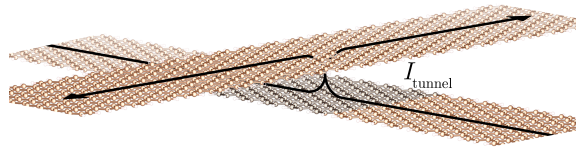
Figure 1. Illustration of an inter-ribbon tunneling structure of two crossed graphene nanoribbons where the inter-ribbon separation has been exaggerated for clarity.. Current flows from one ribbon by tunneling in the overlap region, as indicated. The depicted ribbons have an armchair edge and are only 2 nm wide.
