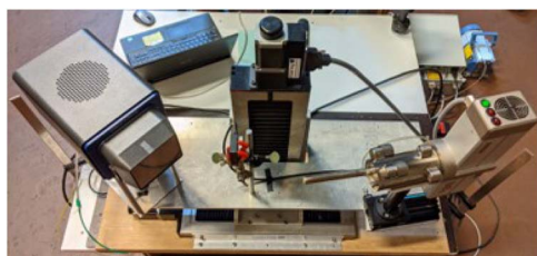
Fig. 4 Image of the scanning XRD setup.
