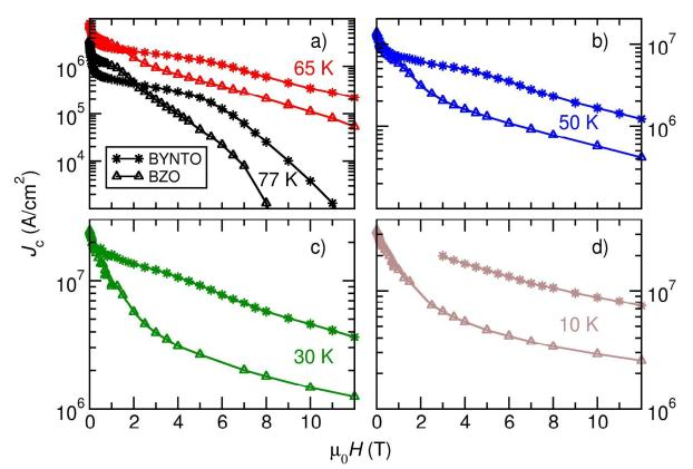
Figure 3:  $J_c(B)$  comparison for ENEA YBCO-BYNTO (stars) and ENEA YBCO-BZO (triangles) in the temperature range [10-77] K. Both systems were grown under conditions optimized for  $J_c$  and  $T_c$  at 77 K.
