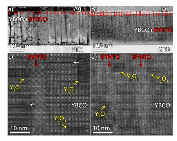
Figure 6: Cross-section overviews and high resolution HAADF STEM images of the 1 Hz (a, c) and 10 Hz (b, d) YBCO-BYNTO films. BYNTO columns are marked by red arrows. Note the higher density of columns in the 10 Hz sample. The samples are highly decorated by  $Y_2O_3$  nanoparticles (~1-20nm). The white arrows indicate double CuO chain plane intergrowths in the YBCO matrix.
