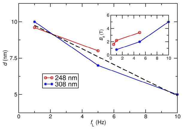
Figure 7: Experimental diameter of the nanocolumns as a function of the laser repetition rate (stars refer to  $v_L$  = 308 nm, circles refer to  $v_L$  = 248 nm) and corresponding linear fit (dashed line). The inset shows the behaviour of the matching field as a function of the laser repetition rate.
