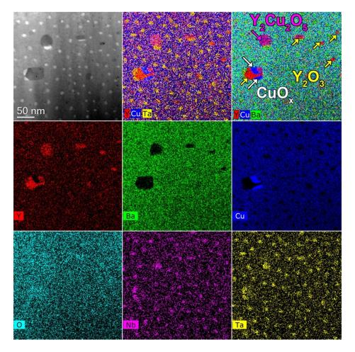
Figure 5: Plan view HAADF STEM image of a film grown at  $f_L = 1$  Hz, with energy dispersive X-ray maps (EDX) showing the elemental composition. Homogeneously dispersed BYNTO columns intersecting the film plane are observed.
