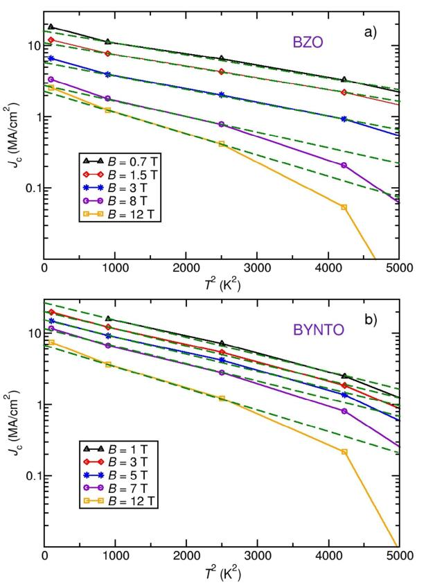
Figure 8:  $J_c(T)$  on log scale vs  $T^2$  at various magnetic fields values for YBCO-BZO (a) and YBCO-BYNTO (b) films. Green dashed lines are data fits according to the empirical formula  $J_c(T) \sim J_c(0) \exp(-3(T/T^*)^2)$ .
