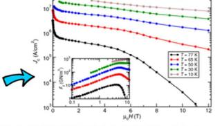
Tailoring of self-assembled nanoinclusions in the YBCO matrix improves in-temperature and in-field performances
