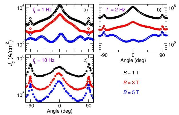
Figure 4: Influence of the laser repetition rate on the angular dependence of  $J_c$  at 77 K and applied field values 1 T, 3 T and 5 T. Zero degrees corresponds to the field orientation parallel to the YBCO c-axis.
