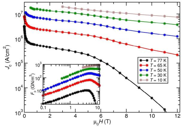
Figure 1: Dependence of the critical current density  $J_c$  on the applied magnetic field up to 12 T (B|/c) of the ENEA YBCO-BYNTO film in the temperature range [10 – 77] K and corresponding pinning force densities  $F_p(B)$  (inset). The slopes of these  $F_p$  curves correspond to 1- $\alpha$ .
