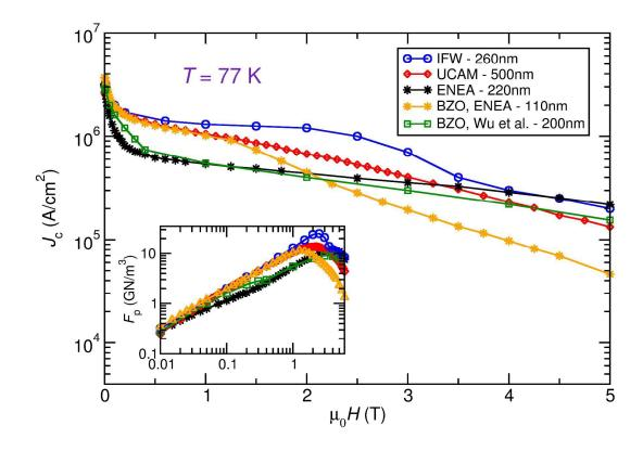
Figure 2: Comparison of the magnetic field dependence of the critical current density at T = 77 K for B|/c of YBCO-BYNTO grown by different groups, IFW (blue circles), UCAM (red diamonds) and ENEA (black stars), as well as high-quality YBCO-BZO films (Wu et al. [17] green squares and ENEA orange triangles). Inset: corresponding pinning force densities  $F_p(B)$ .
