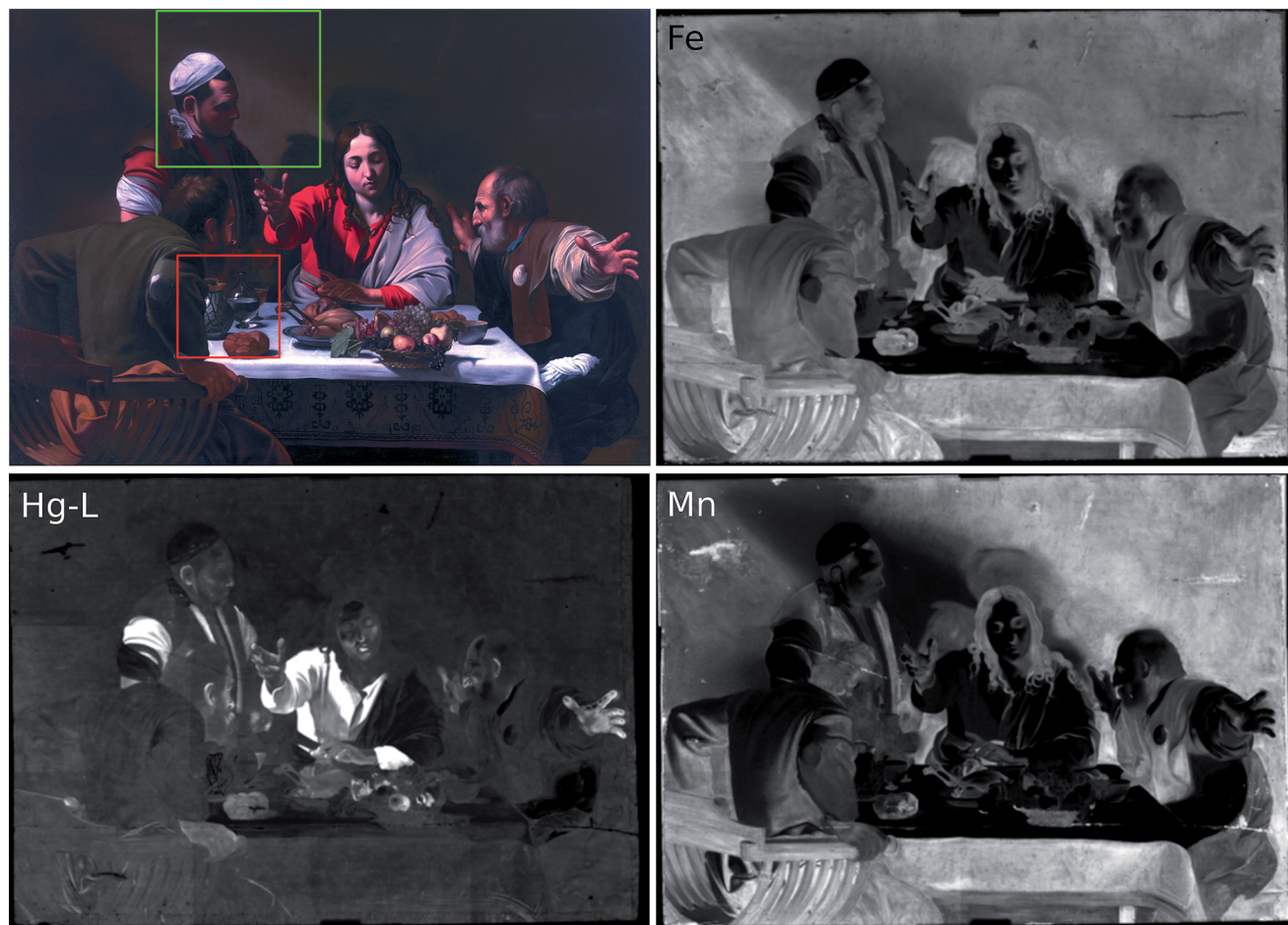
Fig. 1 Supper at Emmaus (143 × 199.5 cm 2 , oil and tempera on canvas), private collection. Photograph and elemental distribution images of Mn, Fe and Hg. The red and green shapes indicate the areas discussed in detail in Fig. 3 and 8, respectively. Data processed with the in-house written software (datamuncher).
