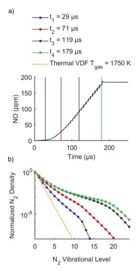
Fig. 5 (a) Calculated NO concentration (black curve) as a function of time, during its residence time in the plasma (at  $1 L \min^{-1}$ ), encountering a train of pulses, and (b) calculated VDF of  $N_2$  taken in the middle of each pulse, for four different time points, as indicated by the vertical coloured lines in (a). The thermal VDF at 1750 K is also plotted.
