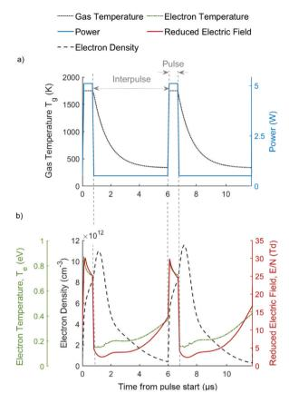
Fig. 3 (a) Input plasma parameters in the model, i.e., gas temperature and power for two pulses. (b) Calculated plasma characteristics, i.e., electron temperature, electron density and reduced electric field, as calculated in the model, for air composition (80/20 N<sub>2</sub>/O<sub>2</sub>) and feed gas flow rate 1 L min<sup>-1</sup>. The vertical grey dashed lines indicate the pulse and interpulse times.
