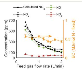
Fig. 4 NO, NO<sub>2</sub> and total NO<sub>x</sub> (dashed lines) concentration as measured by FTIR, calculated total NO<sub>x</sub> concentration (black; full line) and measured EC (orange; right y-axis) as a function of the feed gas flow rate. Error bars are plotted but are barely visible at most flow rates.
