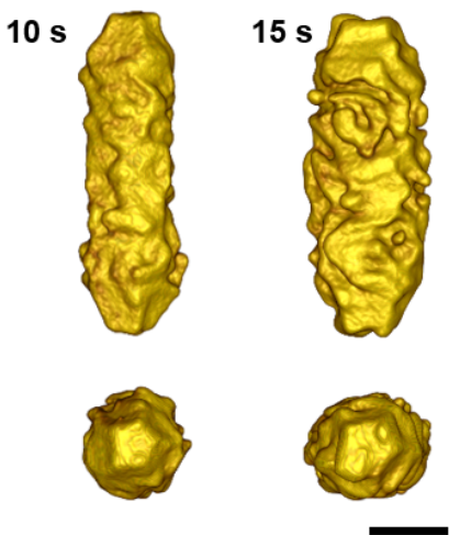
Figure S8. Additional electron tomography reconstructions for the kinetic series shown in Figure 4 of the main text. Nanoparticles were isolated from a chiral growth reaction with penta-twinned Au NR seeds and S -BINAMINE by \text{NaBH}_4 addition after 10 and 15 s. The scale bar is 25 nm.
