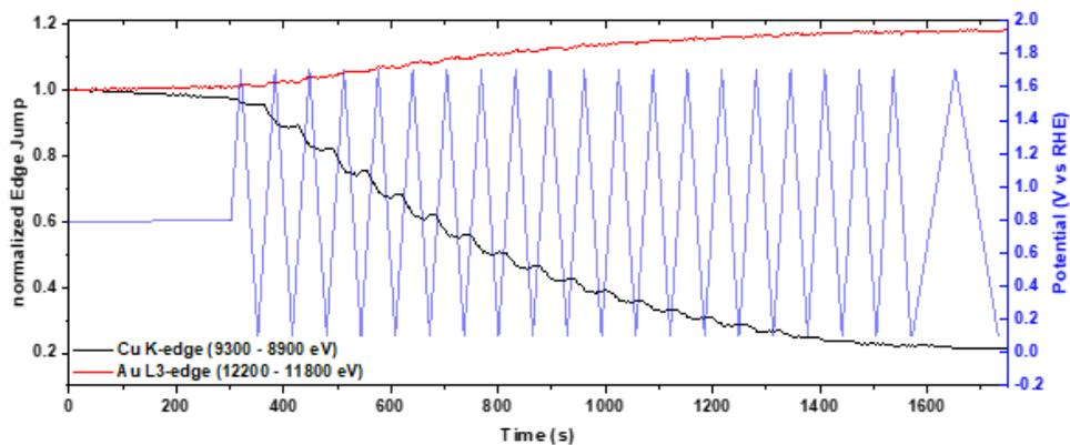
Figure 5. *Operando* normalized Cu K-edge (black line) and Au L<sub>3</sub>-edge jump (red line) during the CV treatment of a AuCu working electrode with a loading of 100  $\mu\text{g}_{\text{catalyst}}/\text{cm}^2$  in CO<sub>2</sub>-saturated 0.5 M KHCO<sub>3</sub> where one datapoint corresponds to an average of 6 spectra. The potential variation over time is depicted as a blue line.
