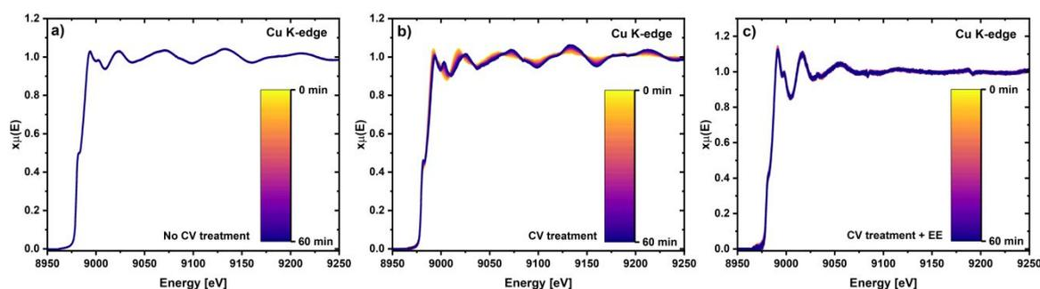
Figure 7. *Operando* GIXAS spectra at the Cu K-edge for a  $100 \mu\text{g}_{\text{catalyst}}/\text{cm}^2$  AuCu aerogel working electrode in CO<sub>2</sub>-saturated 0.5 M KHCO<sub>3</sub> at  $-0.5$  V vs. RHE for 60 minutes undergoing a) no CV treatment, b) CV treatment or c) CV treatment + EE prior to the potential hold.
