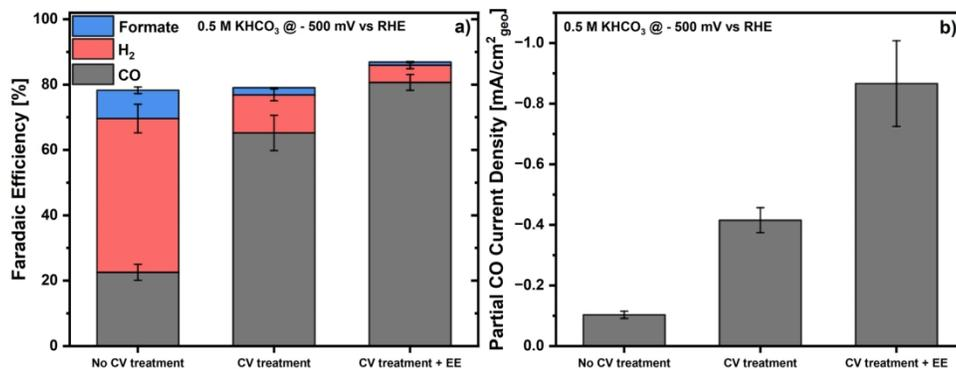
Figure 6. a) FEs for CO, H<sub>2</sub> and formate production and b) partial CDs for CO during the electrochemical reduction of CO<sub>2</sub> in CO<sub>2</sub>-saturated 0.5 M KHCO<sub>3</sub> for a 100 μg<sub>catalyst</sub>/cm<sup>2</sup> AuCu aerogel working electrode undergoing No CV treatment, CV treatment or CV treatment + EE prior to the potential hold at - 0.5 V vs. RHE.
