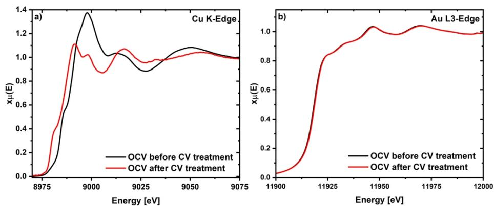
Figure 3. Comparison of the operando XAS spectrum at the a) Cu K-edge and at the b) Au L<sub>3</sub>-edge at OCV before and after the CV treatment of a AuCu Aerogel working electrode with a loading of 100  $\mu\text{g}_{\text{catalyst}}/\text{cm}^2$  in CO<sub>2</sub>-saturated 0.5 M KHCO<sub>3</sub>. Each spectrum represents an acquisition time of 150 seconds.
