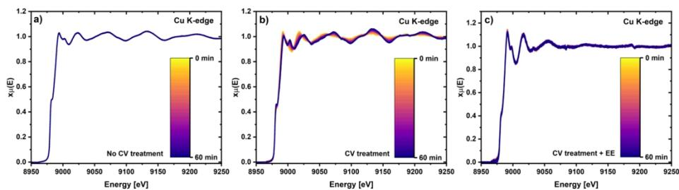
Figure 7. *Operando* GIXAS spectra at the Cu K-edge for a  $100 \mu\text{g}_{\text{catalyst}}/\text{cm}^2$  AuCu aerogel working electrode in  $\text{CO}_2$  in  $\text{CO}_2$ -saturated  $0.5 \text{ M KHCO}_3$  at  $-0.5 \text{ V vs. RHE}$  for 60 minutes undergoing a) no CV treatment, b) CV treatment or c) CV treatment + EE prior to the potential hold.
