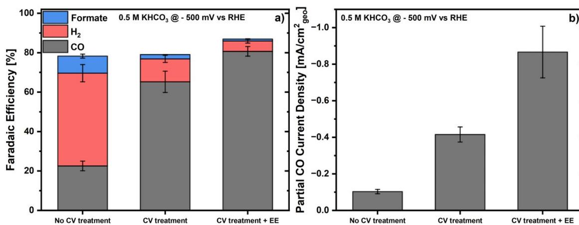
Figure 6. a) FEs for CO,  $\text{H}_2$  and formate production and b) partial CDs for CO during the electrochemical reduction of  $\text{CO}_2$  in  $\text{CO}_2$ -saturated 0.5 M  $\text{KHCO}_3$  for a  $100 \mu\text{g}_{\text{catalyst}}/\text{cm}^2$  AuCu aerogel working electrode undergoing No CV treatment, CV treatment or CV treatment + EE prior to the potential hold at - 0.5 V vs. RHE.
