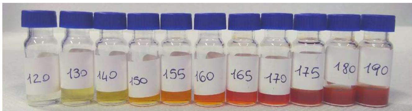
Figure S1. Timeline of the reaction for the synthesis of \text{Pb}_4\text{S}_3\text{Br}_2 NCs by direct observation of aliquots collecting during the synthesis. Many aliquots of the reaction batch were taken using a syringe and immediately quenched by immersing the vial in a water bath. The quenching temperature increases from left to right, as reported in ^\circ\text{C} on each vial.
