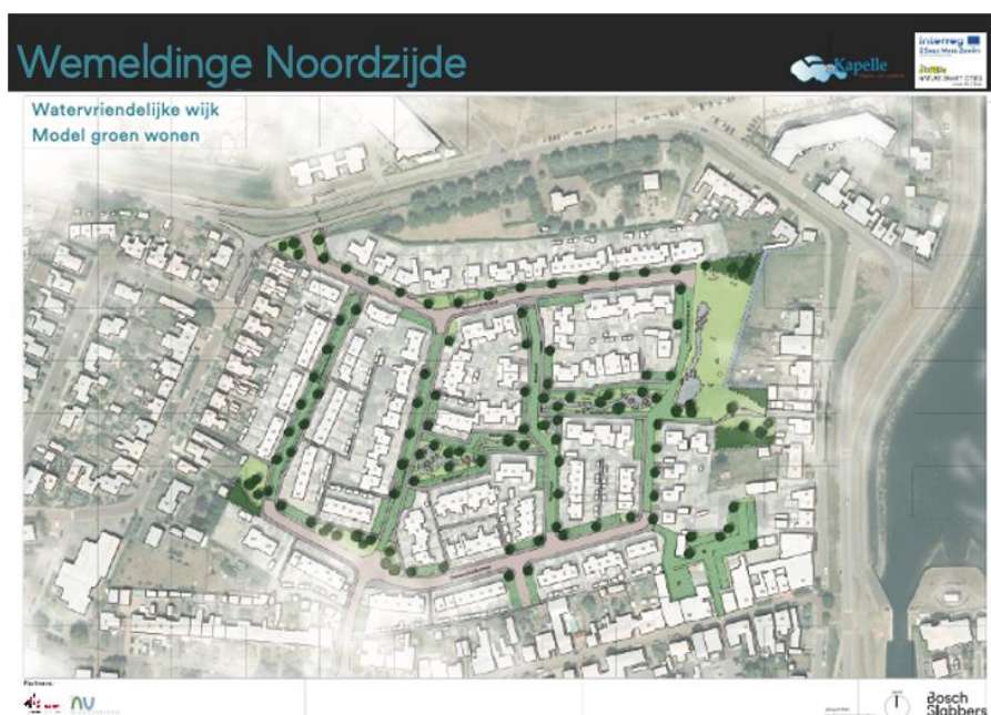
Figure 4: Map of the pilot case project in Wemeldinge Noordzijde, Kapelle. The map shows how the municipality aims to improve local GI provision by making streets (semi-)permeable and by enhancing the design of existing green space.
