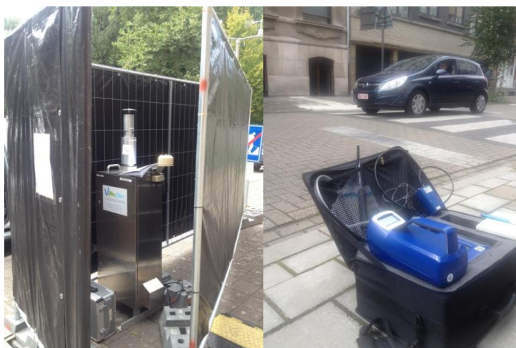
Figure 2: Left: On-site fencing, meteorological mast and monitoring equipment for the continuous gravimetric \text{PM}_{10} measurements (Leckel SEQ 47/50). Right: Applied portable \text{PM}_{10} (TSI Dusttrak II), UFP (TSI P-Trak) and BC (Aethlabs AE51 microaethalometer) instruments for the point measurement campaigns.
