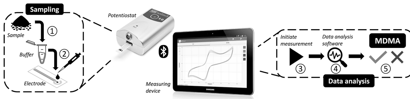
Fig. 1. Sampling and analysis procedure for the electrochemical MDMA sensor.
