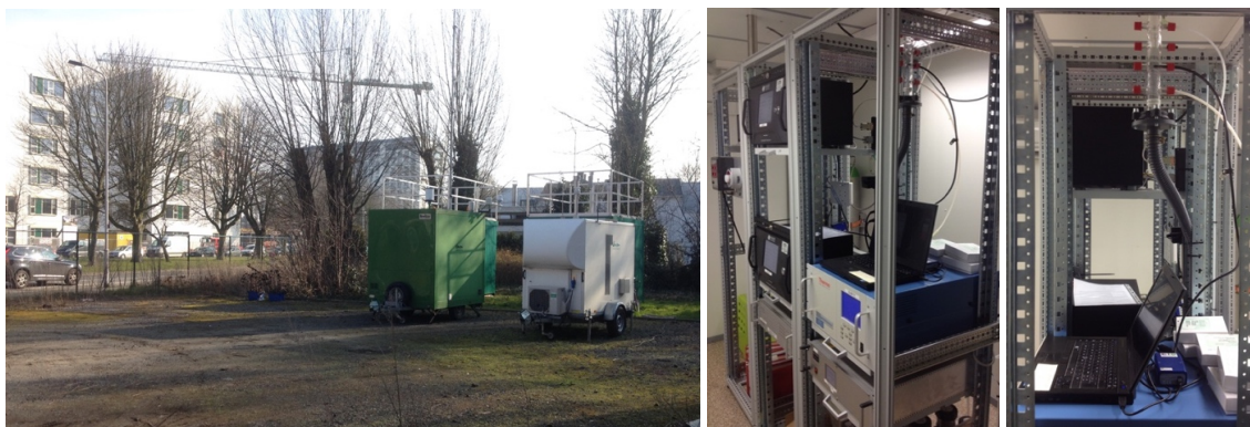
Figure S1: Instrument performance evaluation of the AE51 (attached to laptop), during the 37-hour side-by-side monitoring with the AE33 of monitoring station 42R817 (left picture) of the Flanders Environment Agency (VMM) in Antwerp, Belgium. The sample tubing of both AE51 and AE33 were connected to a similar inlet (right picture).
