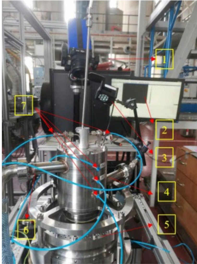
Fig. 2. Photographic view of the STARVOC unit. 1 - PIV camera, 2 - computer, 3 - light, 4 - air inlet, 5 - reactor, 6 - air outlet, 7 - pressure measurement taps.
