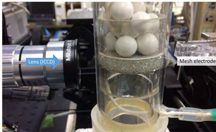
Figure 2: Experimental configuration of the packed bed plasma reactor, used for ICCD imaging.
