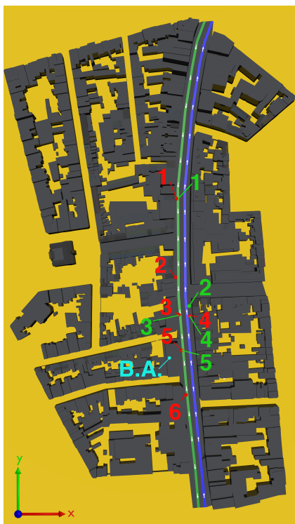
Figure 6: Location and numbering of available experimental data of wind velocity and direction (highlighted in red), and PM_{10} concentration (highlighted in green), in the Turnhoutsebaan. The base anemometer (B.A.) is indicated in light blue, at coordinates ( x = -17m , y = -151m , z = 32.5m ).
