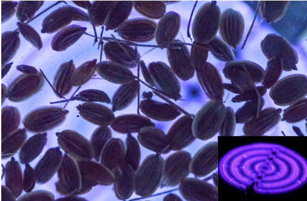
Figure 5: Example for food treatment by non-thermal atmospheric pressure plasma. Dill ( Anethum graveolens ) seeds treated with dielectric barrier discharge (DBD). Small photo: DBD with plasma turned on, ring-shaped electrode configuration. Taken from Schnabel et al. 2017 [85] .
