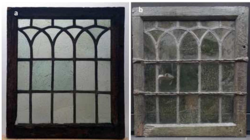
Figure 1. The exterior side of the leaded window (a) in transmitted light and (b) in reflected light.
