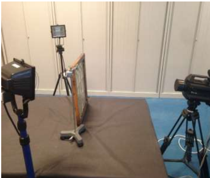
Figure 5. Transmission set-up for the IRT measurements with the back of the window heated. In reflection mode, the window is heated from the front side with the lamps alongside the camera while maintaining the same distances and angles with respect to the window.
