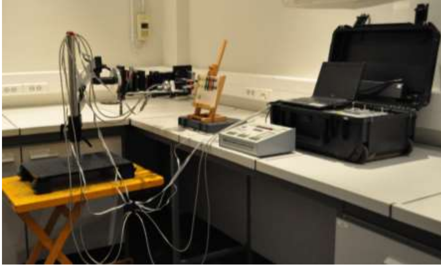
Figure 4. The portable EZRaman-I dual spectrometer. Two different excitation probe heads are attached to the articulated arm for easy positioning and focusing of the beam. Credits: Debbie Lauwers.
