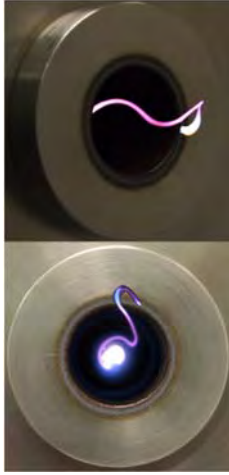
Figure 10. Photos of the outlet of the GAP (anode), showing the arc discharge. The arc is stabilized in the middle of the reactor, where it is attached to the cathode and anode.
